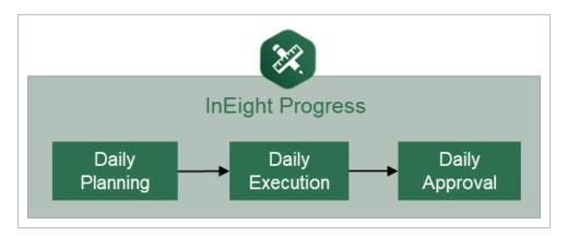
A daily plan is created by a project member to specify the tasks to be completed by a given crew, and to ensure productivity targets are met. Budget, quantity, safety, quality and other details are entered during the Planning phase to provide streamlined communication from the office to the field. Once the planner, typically a superintendent, field engineer or indirect supervisor is satisfied with the daily plan details and planned productivity, they will submit the plan to the Execution Phase.
