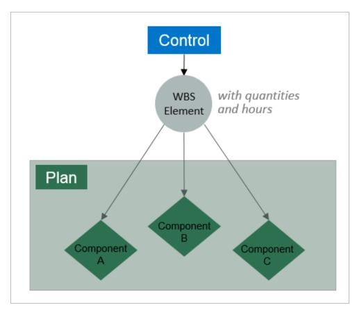
In Eight Progress uses the component quantities along with actual hours to determine productivity.
